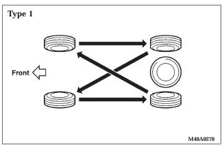
To equalize wear and help extend tire life, the manufacturer recommends that you rotate your tires approximately every 7, 500 miles (12, 000 km) under normal driving conditions and every 6,000 miles (9,600km) in severe driving conditions.
